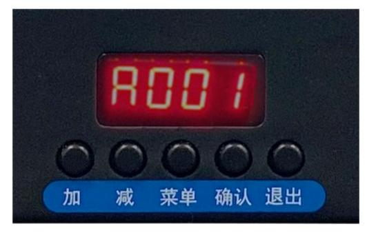
Control the start address of the dmx512 channel by addition and subtraction
